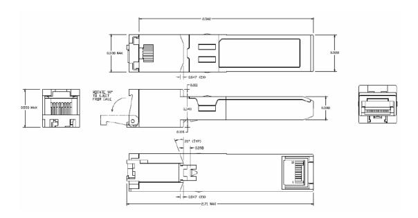
Figure 2. mechanical dimensions
