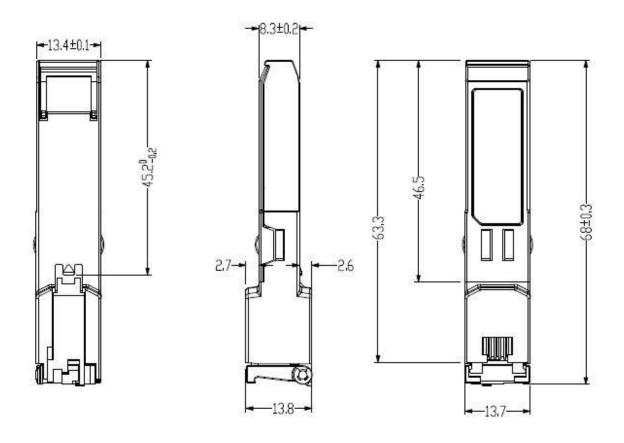
Figure 2. Mechanical Dimensions of Transceiver
