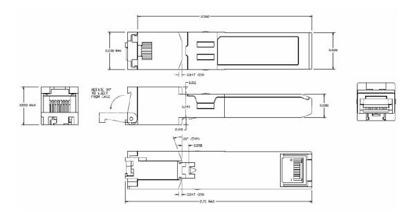
Figure 2. mechanical dimensions
